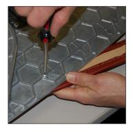
Attach palm rest to, or remove it from, the aluminum tray with the 2 Phillips-head screws that secure it from the underside of the tray. Installing Tray to Arm
