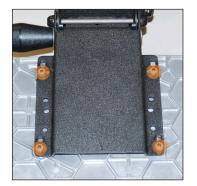
Position the tray over mechanism/arm so the pre-installed bolts in the tray line up with the holes in the arm mounting plate. Install and tighten a lock washer with a <sup>3</sup>/<sub>8</sub>" nut on each of the threaded bolts to secure it to the mounting plate.
