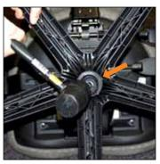
2. Wearing safety glasses, hold one leg of the base (gloved hand recommend) and strike the cylinder protruding through the base, using a plastic or rubber hammer in your other hand. The force will
