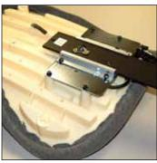
Replace with new assembly and install with the 4 screws previously removed.
