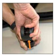
4. Grasp base with one hand (gloves suggested) and pull caster out with the other. Repeat on each leg. If any are stuck, you can pry it out using a flat screwdriver.
