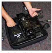
Replace with the new mechanism and attach to the seat by inserting screws previously removed.
