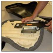
Lift the back to the highest setting to remove tension from the spring.
