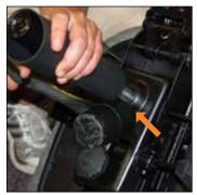
4. Firmly holding the cylinder with one hand, use hammer to strike the mechanism around the cylinder entry point.\*\*
