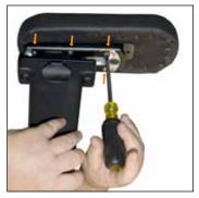
To reduce resistance/ friction, loosen the 6 Phillips-head screws located along the bottom of the tracker piece.
