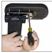
To tighten the resistance/ friction of the tracker piece, tighten the 6 Phillips-head screws located along the bottom of the tracker piece. You may will need to slide the tracker to gain access to the middle screws.
