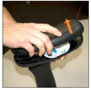
Remove pad, keeping the screws handy for reinstallation.
