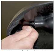
Attach the lumbar pillow air hose to the nipple of the bulb reinstalled in step 4.
