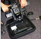
Lift the mechanism off the seat from the rear.
