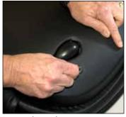
Tighten the screws using the 5/32" Allen wrench, being care to NOT overtighten.
