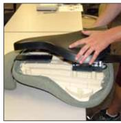
Replace the back shell on the backrest, making sure that the air lumbar hose is still connected.
