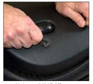
Using a 5/32" Allen wrench, remove the screws securing the outer shell to be replaced from the
