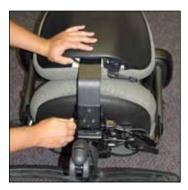
1. Remove the 3 screws (3/16" Allen-head) that secure backrest post to the mechanism. Once detached, place on a clean work surface with the outer shell up and accessible.
