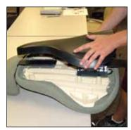
1. Remove the back shell from the backrest portion of the chair. If a 6000/7000 or Big & Tall back, be careful not to disconnect the air hose from the air bulb and valve. (Refer to "Back Outer Replacement" sheets for guidance.)
