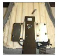
Remove four 3/8" Allen heads bolts securing the aluminum sleeve to the pressure plate.
