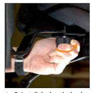
Reinstall the hand wheel with washers in place (lock-washer on first, then beveled washer with concave side down) and tighten at your desired width setting.
