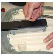
Start the four 5/32" Allenhead screws and tighten to secure the new headrest bar to the internal height adjuster.
