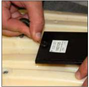
Stretch spring to reach keeper on the JBU and slide over head.
