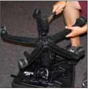
cylinder by firmly holding onto one of the legs of the base and tapping on the bottom of the cylinder with a plastic or rubber
