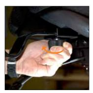
Loosen and remove the handwheel which secures the arm in the bracket under the seat. Keep washers in same order for reinstallation.
