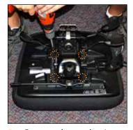
Remove the mechanism from the seat pan by removing the 4 screws (or bolts depending on the model). Use a screw driver if the seat is a 4, 5 or 7 which was manufactured after Sept. 1998 or a 6 manufactured after Apr. 2000. If your chair has been manufactured before Sept. 1998, the seat is held in place with nuts and washers and will require a 7/16" deep socket and ratchet. If not, use a 3/8 socket.
