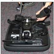
Remove the cylinder from the mechanism by firmly grasping in one hand and using a hammer to tap on the flat surface of the mechanism close to where the cylinder is joined to the mechanism until it comes apart.\*\* This may take several blows.
