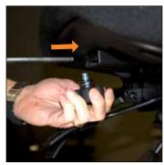
Install the replacement arm in the bracket. The right arm will have the pullout adjustment guide in the arm pad.
