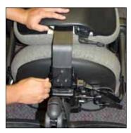
8. With new back shell attached, reattach the back assembly with 3/16" Allen-head screws in reserve steps from Step 1 above.
