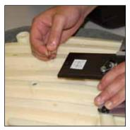
Reinstall spring per instructions. (Refer to Extension Spring Replacement/Height Adjuster sheet.)
