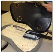
Position and install the new back shell by aligning the tabs with receiving bosses.
