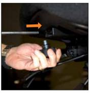
Slide arm assembly back into the bracket.
