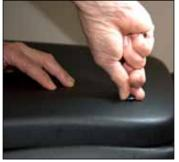
Avoid cross threading the screws by starting them by hand. You may need to locate the screw holes with a thin screwdriver to align them.
