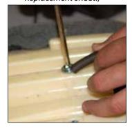
Insert the screw with washer into keeper ring of the new spring and reaffix to the back in the same hole.
