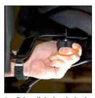
8. Reinstall the hand wheel with washers in place (lock-washer on first, then beveled washer with concave side down) and tighten at desired width setting.
