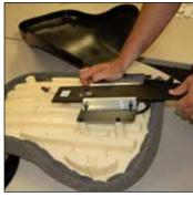
Lift the back to the highest position on the back bar to eliminate tension from the spring.
