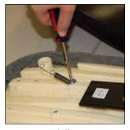
Using a Phillips screwdriver, remove the screw and washer holding the opposite end of the spring.
