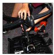
Replace the cylinder and base assembly by placing the cylinder into the mechanism and pressing firmly.
