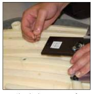
3. Slip the lower spring from the retainer on the JBU (i.e. back post).
