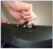
Pull the air hose from the nipple of the air bulb.
