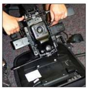
5. Lift the mechanism off the seat pan from the rear.
