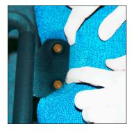
To remove the fully upholstered backrest, locate the 4 (⅔2") Allen-head bolts where the frame attaches to the backrest. You'll need to pull back the edge of the upholstery on the outer shell to access those bolts. Remove the 2 bolts on each side of the backrest.
