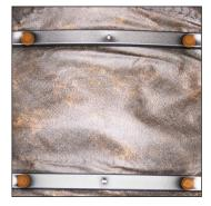
To remove the seat, access the underside and locate and remove all 4 (%22") Allen-head bolts.
