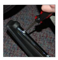
Replace pads in reversed order. Always start screws by hand, being careful not to cross-thread.
