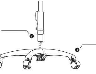
Press casters firmly into base until they are securely snapped into place.
